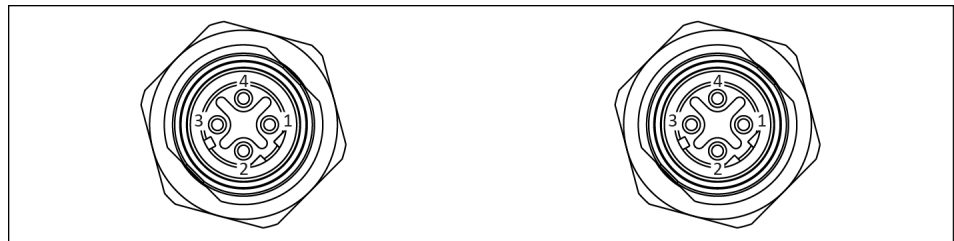
PIN allocation of socket and socket, PROFINET variant
